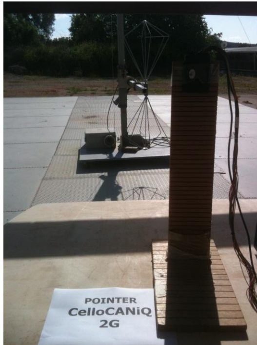
Figure 3 Spurious Emission Test
